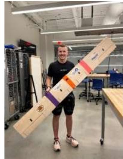
On December 7, 2024, TED-1 flew its maiden flight at Jetway Airport-61OH. Constructed from balsa wood, foam, and 3D-printed PLA, TED-1 featured a 6-foot wingspan and twin KDE Direct 4215XF motors. Although tail-heavy, the aircraft flew successfully under the control of pilot Joshua Shutic.
